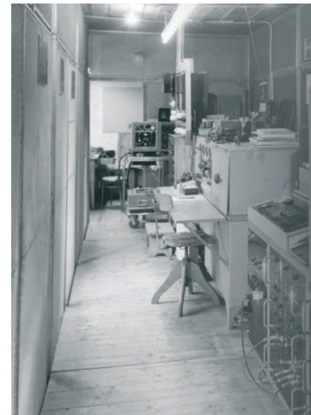
Laboratory within the Faraday-cage we find a high speed Cathode ray oscilloscope in front and low speed mirror-galvanometer-oscilloscope in the middle. Summer 1971
